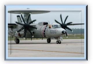
**8. Stoof with a Roof.** The dome-like top piece of the E-2C Hawkeye is used to detect enemy aircraft and ships at great distances plus it has many other important duties. Its unique propeller design helps it perform well in all weather.
